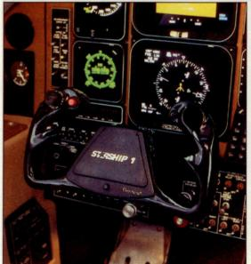
The Starship's futuristic image is reflected in the 16tube Collins instrument panel, designed expressly for the airplane. All navigation and communication information, including frequencies and identifiers, is fed to the black boxes via pilot and copilot keypads. Displays can be transferred among the various tubes. The only mechanical instruments are stand-by attitude and airspeed indicators and an altimeter.
